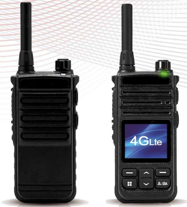
The CP625/CP626 from BTI WIRELESS are a pair of compact and smart PoC two-way radios that offer nationwide (or even worldwide) coverage over 4G/LTE networks for your PTT communications. The user can enjoy license free nationwide radio communications. With a battery capacity of 5200mAh, the CP625/CP626 can easily meet the battery needs of long day operations.
